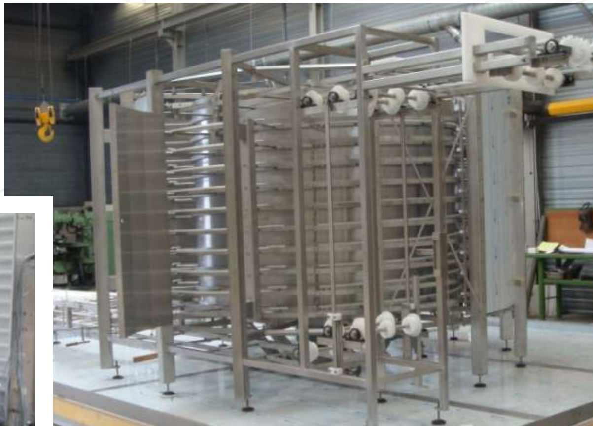
Cooling- and Freezing conveyors.
